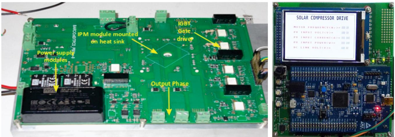
Fig.2: Power board with three leg IGBT Inverter module mounted on heat sink and Signal board with ARM based MCU unit, 3.2" LCD module and user interface.
