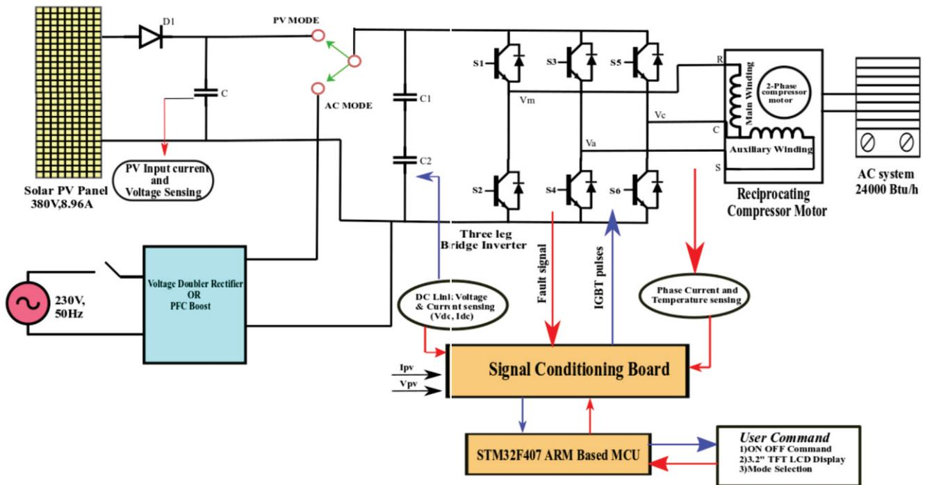
Fig.1: Block diagram of Air conditioning compressor drive powered by both solar power and 1-phase 230V, 50Hz AC supply.
