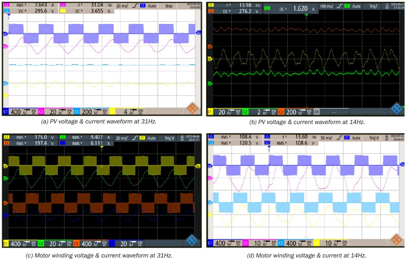
Fig.4: Test waveform at various solar insolation. (a) PV voltage, current main winding voltage & current at 31Hz. (b) PV voltage, current main winding current at 14Hz. (c) Voltage & current waveform at motor windings at 31Hz. (d) Voltage & current waveform at motor windings at 14 Hz.
