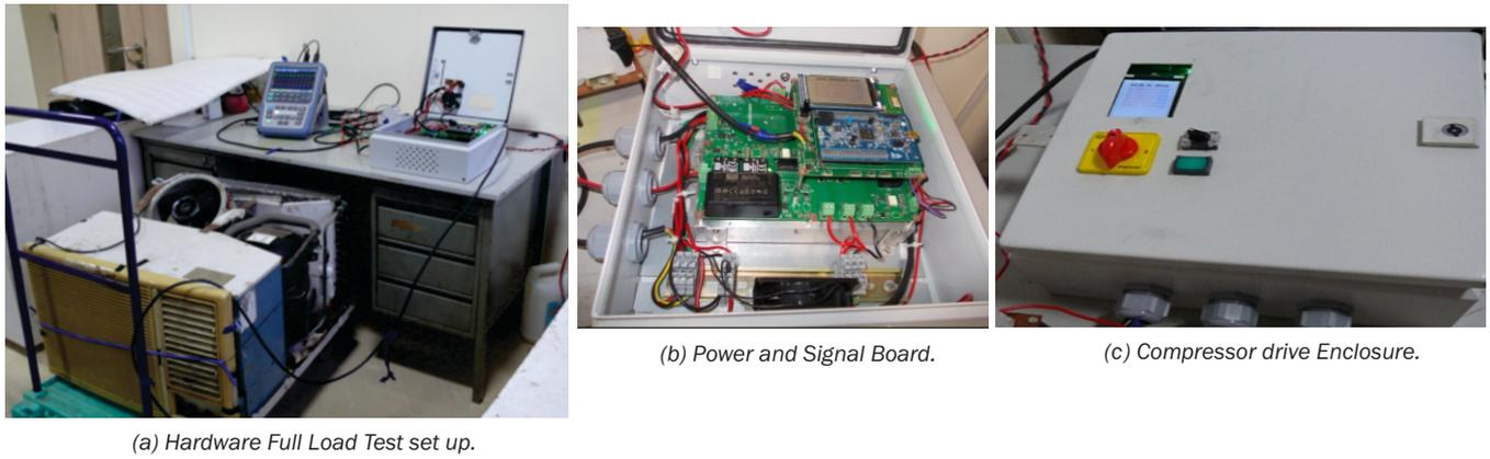
Fig.3: Air conditioning compressor drive powered test setup. (a) Inverter stack powering 2.3kW Compressor motor in 2-Ton AC unit. (b) Powered board and signal board assembled in a 300mm x 300mm x 210mm IP55 housing. (c) Compressor drive system in a wall mounted IP55 metal enclosure.
